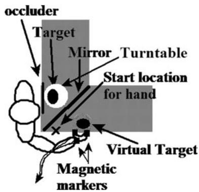
**Fig. 1** Arrangement of the experimental apparatus. See the text for explanation
